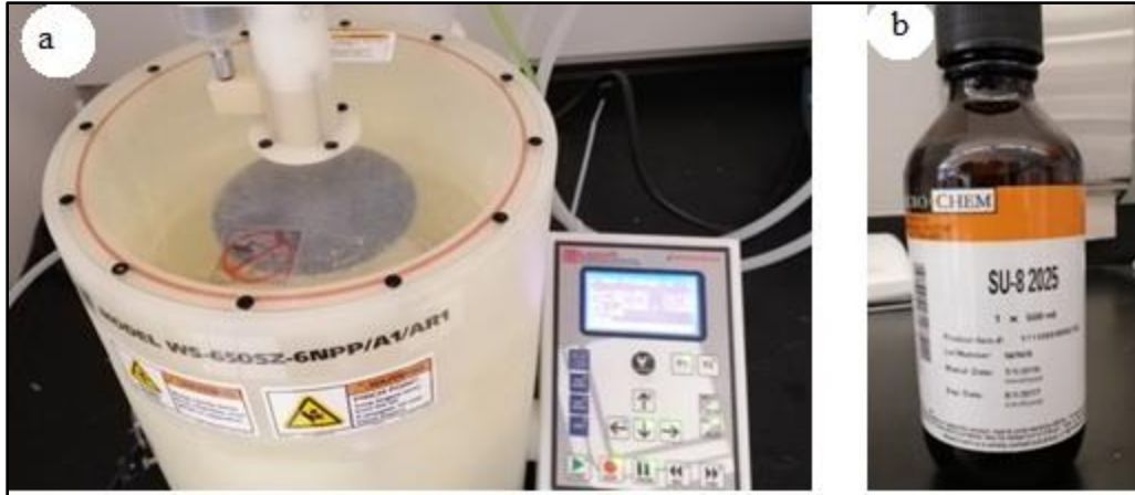
Figure 7: a) Spin coater, b) SU-8 negative photoresist.
