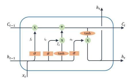
Figure 2. Unit LSTM cell
