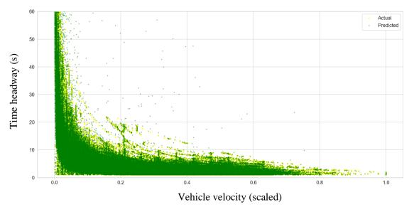
Figure 30. Correlation of vehicle velocity with time headway in I-80 (actual vs predicted)
