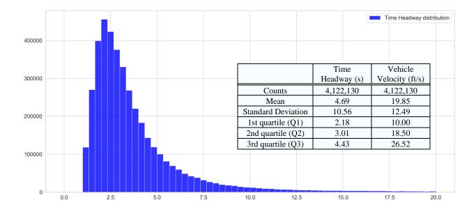
Figure 6. Statistics & distribution of Time Headway (x-axis: time headway, y-axis: counts of headway)
