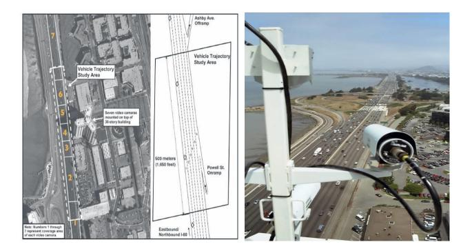
Figure 4. Aerial view of the subject area (left) and a digital video camera mounted on top of a building recording vehicle trajectory data of I-80 (right)
