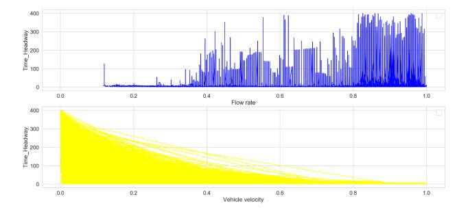
Figure 9. Correlation of time headway with flow rates and velocity
