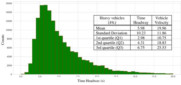
Figure 13. Time Headway distribution of Vehicle Class-3 (truck)
