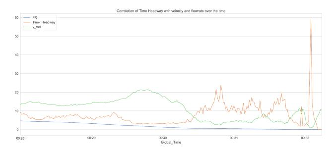
Figure 10. Correlation of headway with velocity and flowrate (last four minutes)
