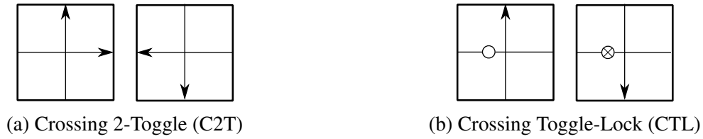
Figure 4.11: (a) The two states of the crossing 2-toggle gadget. Robot traversal through either tunnel toggles the gadget between these two states. (b) The two states of the crossing toggle-lock gadget. Robot traversal through the directed tunnel toggles the gadget between these two states (locked and unlocked).
