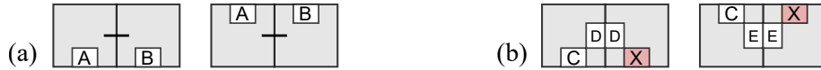
Figure 3.1: The black lines between two tiles indicate unique unimportant \tau -strength bonds. If \tau = 2 , str(A) = 1 and str(B) = 1 , then the two assemblies in (a) are \tau -combinable, since str(A) + str(B) \geq \tau and the positioned assemblies may be translated such that the A and B glues are aligned—such a combination is termed cooperative binding , since neither the A nor B glue are alone sufficient to satisfy \tau -combination. In (b), we consider two cases concerning the negative strength glue X . If \tau = 2 , str(C) = 2 , and str(X) = -1 , then the assemblies in (b) are not \tau -combinable since str(C) + str(X) < \tau . If \tau = 1 , str(C) = 2 , str(D) = 2 , str(E) = 1 and str(X) = -1 , then the assemblies are \tau -combinable since str(C) + str(X) \geq \tau ; however, the resultant assembly is unstable, since a cut along the X and E glue has strength str(X) + str(E) < \tau ; this violates the valid growth-only system definition.
