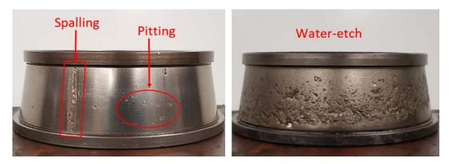
Figure 3. Example of localized defects (left) and distributed defect (right)
