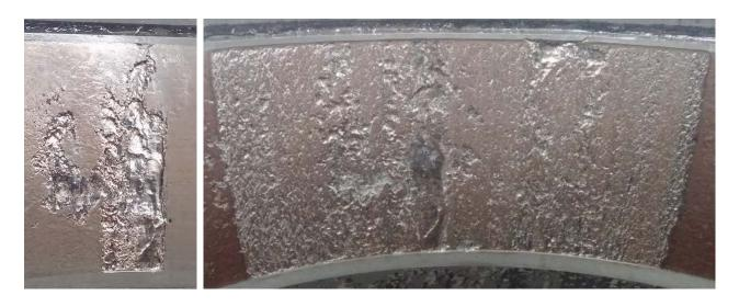
Figure 33. Experiment 184B: Initial cup raceway (left) and final cup raceway (right)
