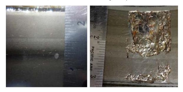
Figure 30. Experiment 200: Initial cup raceway (left) and final cup raceway (right)
