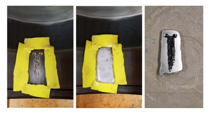
Figure 17. Casting procedure using sealant and bismuth tape
