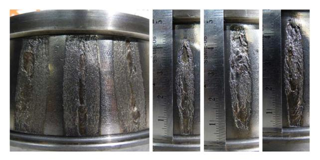
Figure 39. Experiment 206 initial cone raceway (multiple spalls)
