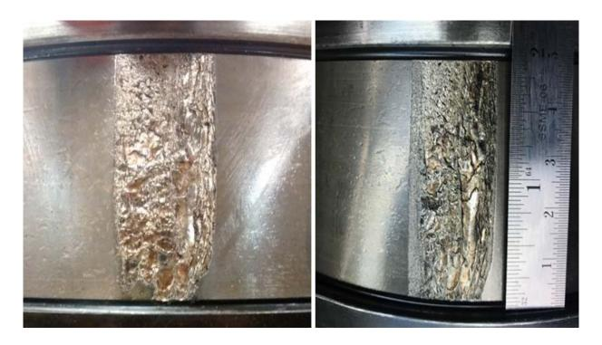
Figure 36. Experiment 202A: Initial cone raceway (left) and final cone raceway (right)
