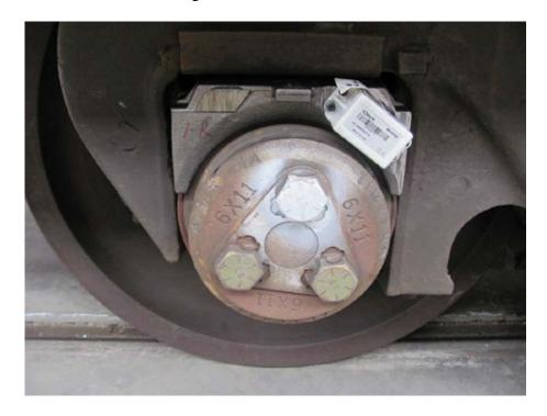
Figure 7. Field installation of a Wireless Sensor Node
