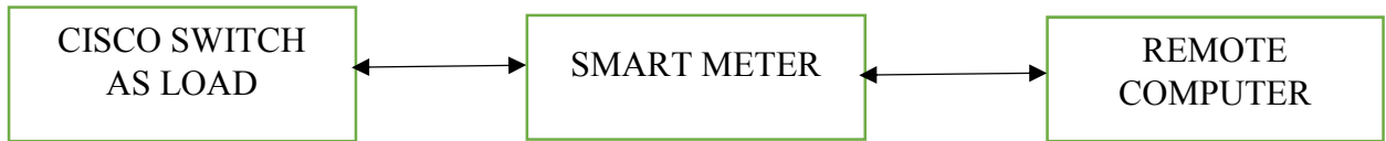
Figure 2.10: Experimental set up to monitor WH consumption of switch as a load
