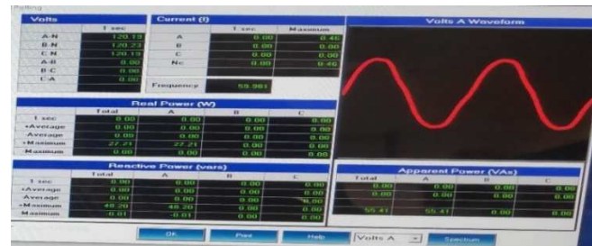
Figure 4.1. Smart Multifunction Meter (EPM 7000) with Ener Vista Software for remote power recording from GE [55]
