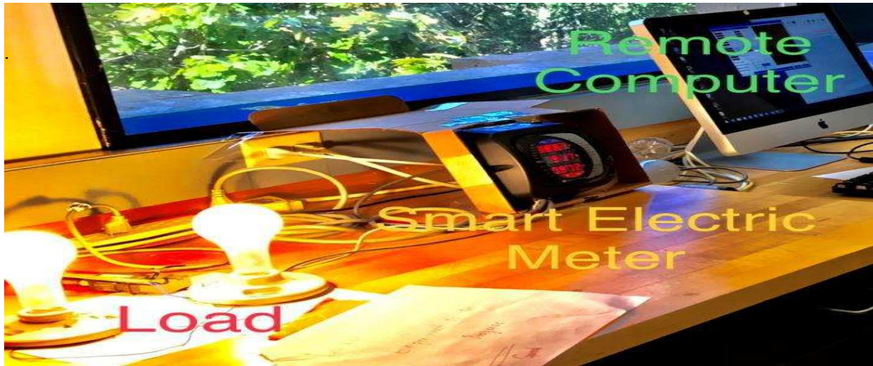
Figure 3.5: Lab set up used in Experiments showing Load, Smart meter and monitoring remote computer [41]
