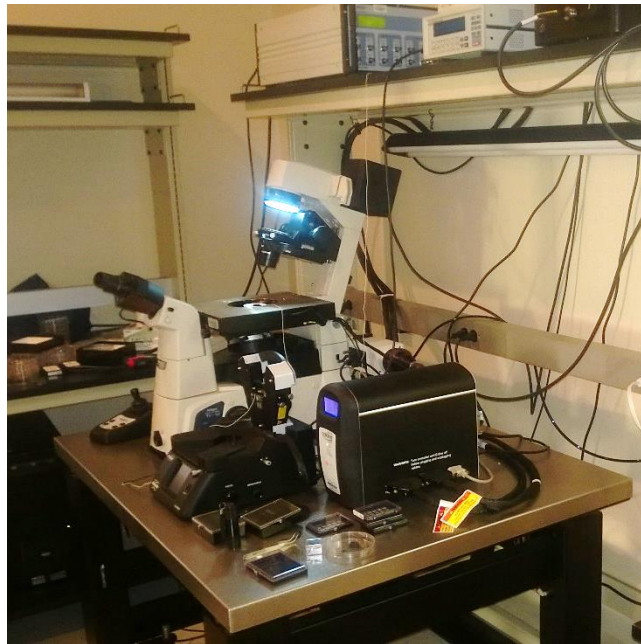
Figure 5. Bruker Bioscope Atomic Force Microscope used in the present study. The AFM is combined to an inverted fluorescence microscope
