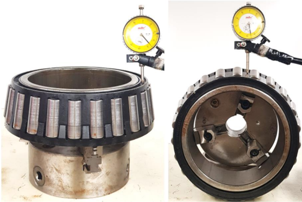
Figure 12. Inner ring (cone) assembly measurements: cage lift (left) and cage shake (right)
