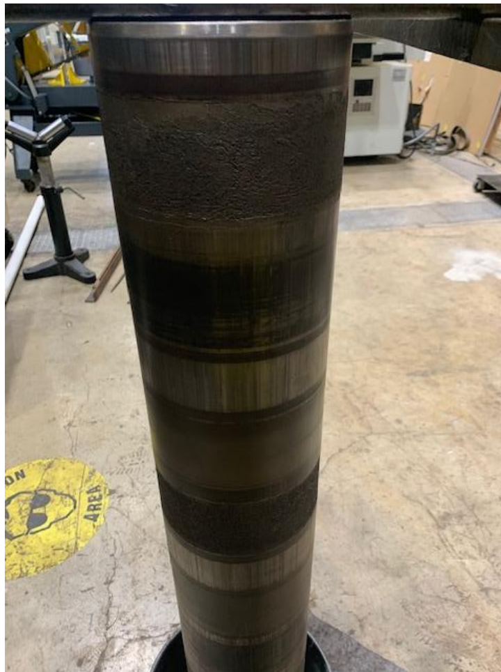
Figure 30: Experiment 225 axle damage
