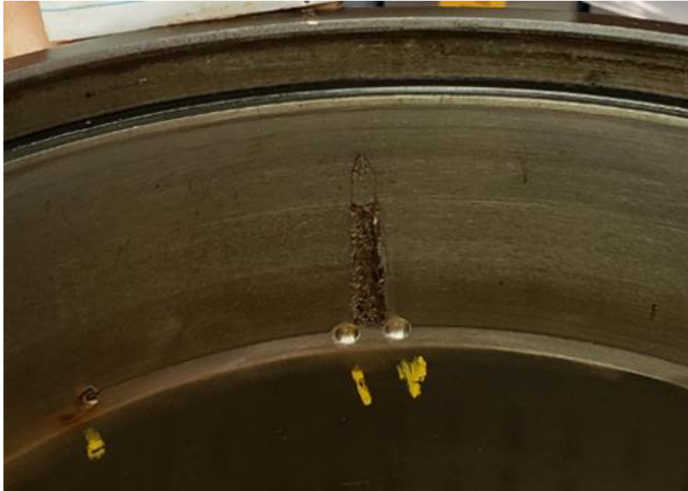
Figure 25: A picture of the defect that developed on test bearing 2 (B2) after 151,154 km (93,923 mi) of total operation since the bearing was reconditioned
