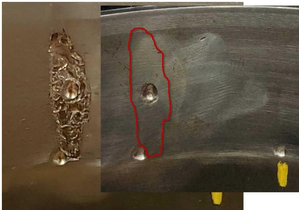
Figure 27: A picture of the defect that developed on test bearing 3 (B3) after 14,001 km (8,700 mi) of total operation since the bearing was reconditioned
