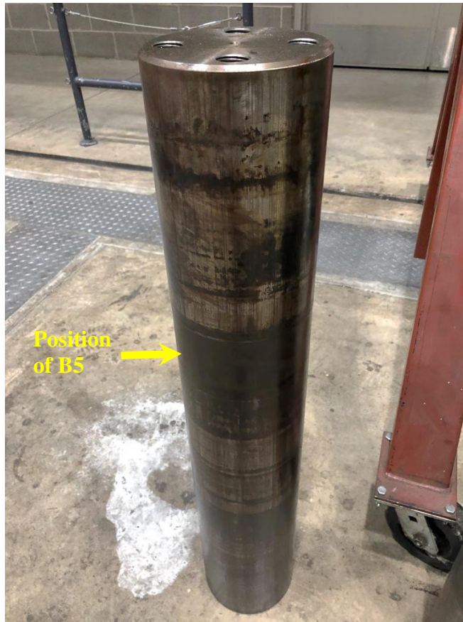
Figure 43: Experiment 229C axle damage
