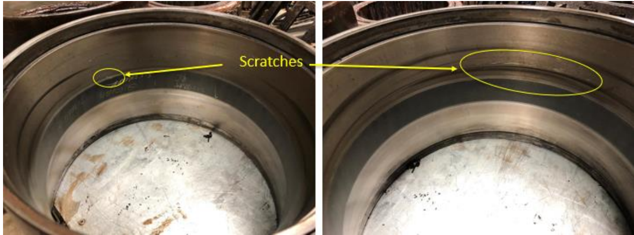
Figure 38: Damage on cup raceways of test bearing 6 (B6)
