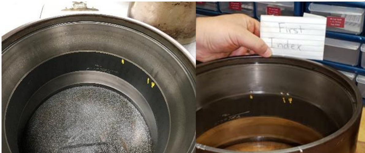
Figure 19: Picture on the left side shows test bearing 2 (B2) before the reconditioning process. The picture on the right shows test bearing 2 (B2) after it was reconditioned with the “Index I” region shown.
