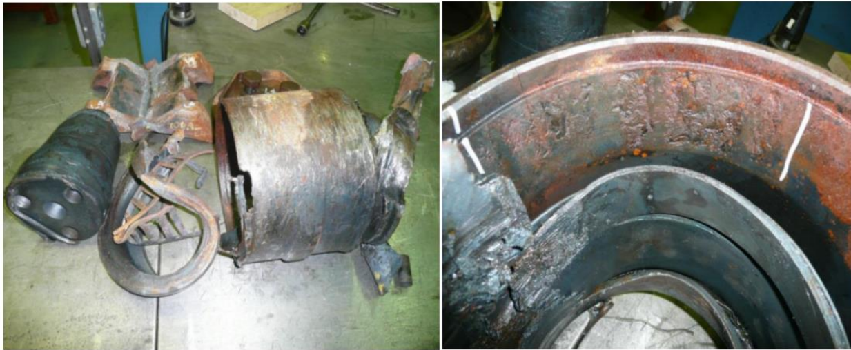
Figure 8. Burnt-off journal from railcar SKPX 622514 [16]
