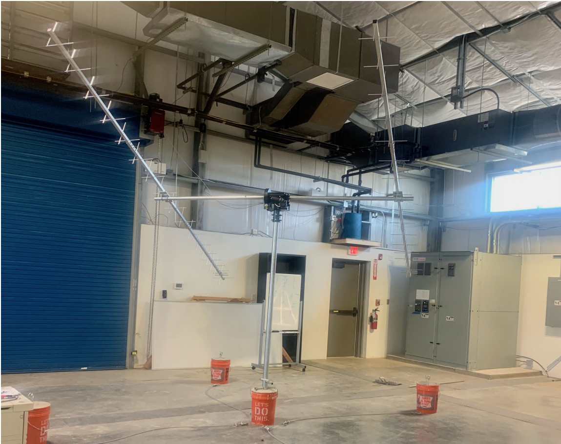
Figure 3.1: Showing a pair of antennas attached to a cross-boom, mounted on a BigRAS rotator, cemented in a concrete bucket, the supporting guy wire, and respective mounting points.
