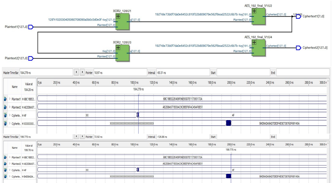
Figure 119: Timing Simulation For AES-192 in CBC Mode
