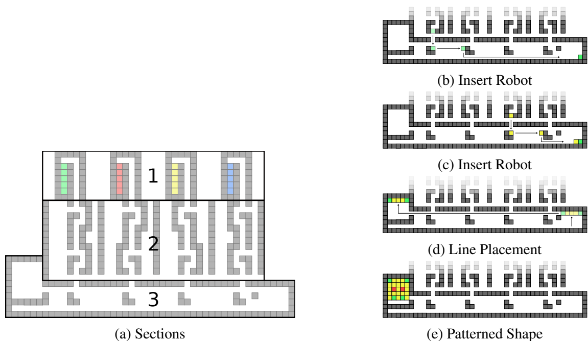
Figure 4.7: An overview of the k -color constructor for k = 4 . (a) This is a 4-color pattern constructor in its starting configuration. (b) We refer to various sections of the configuration by different names. Section one is the fuel chamber , section two has the bit string gadgets, and section three is the line and construction chamber .
