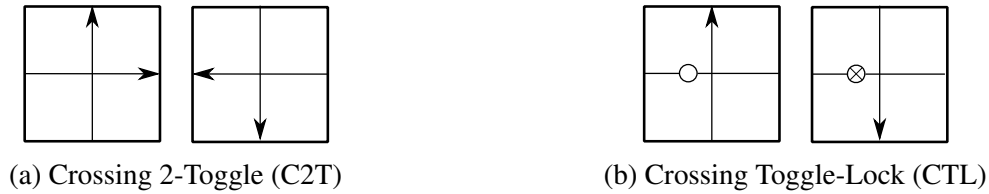
Figure 5.1: (a) The two states of the crossing 2-toggle gadget. Robot traversal through either tunnel toggles the gadget between these two states. (b) The two states of the crossing toggle-lock gadget. Robot traversal through the directed tunnel toggles the gadget between these two states (locked and unlocked).
