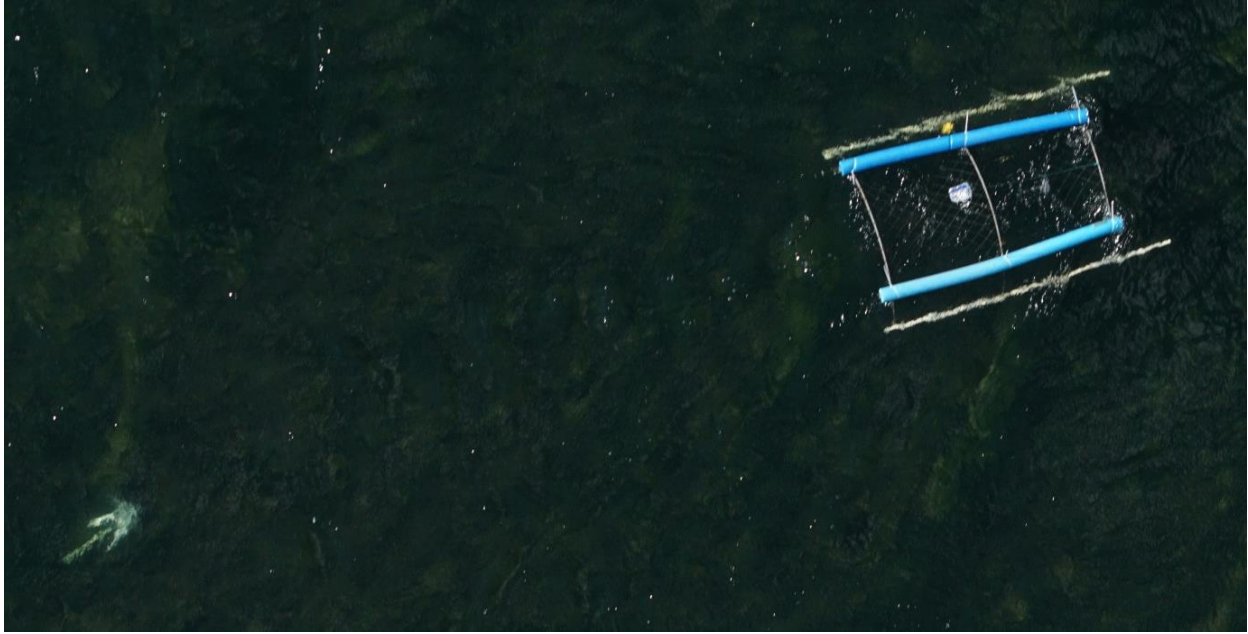
Figure 9. Floating trap deployed in sampling area. On the right, the trap, PVC piping (white), pool noodles (blue), and bait can are visible. On the bottom left, the anchor is visible under water. These traps were successful at trapping turtles in locations where habitat characteristics prevented the securement of baited hoop-net traps to shore or where water levels fluctuated due to variable releases from upstream dams.
