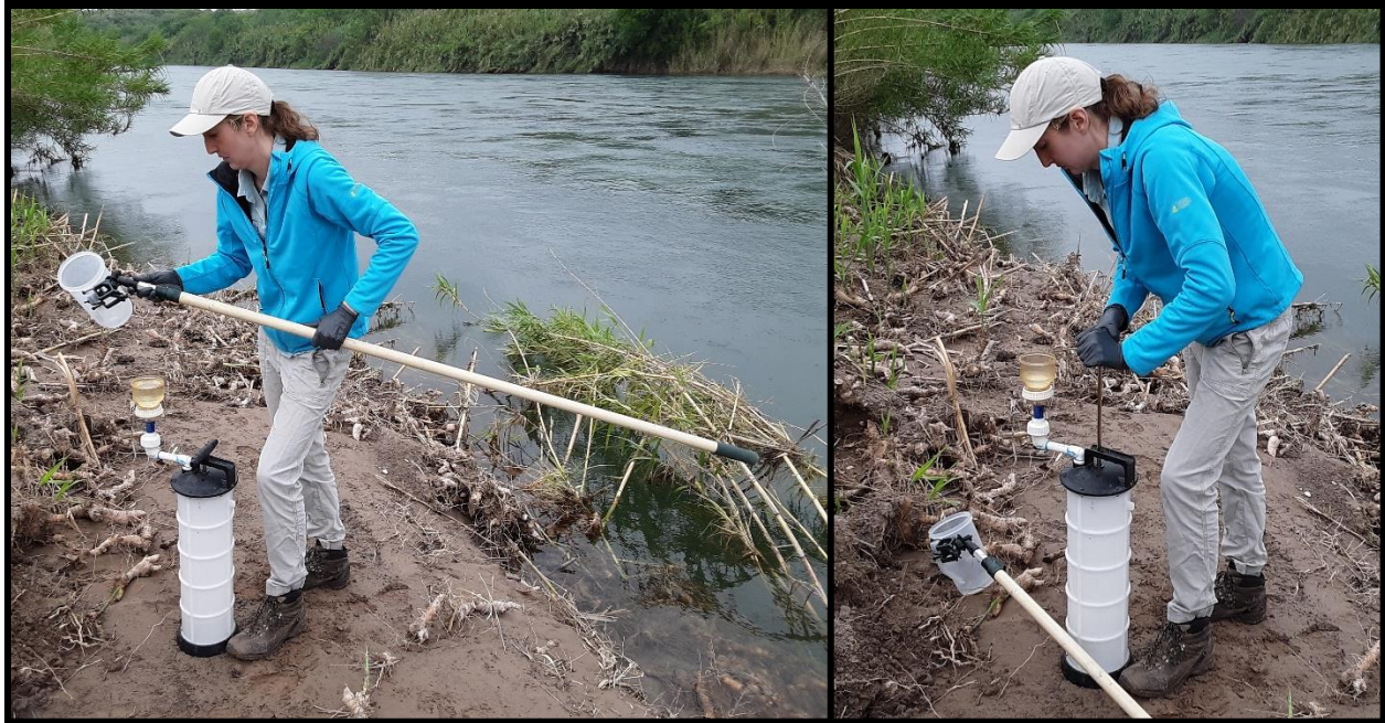
Figure 23. Equipment used to acquire environmental DNA (eDNA) samples. This includes the plastic pitcher, telescoping sampling pole, 47-mm filter cup, and hand-powered fluid excavator.
