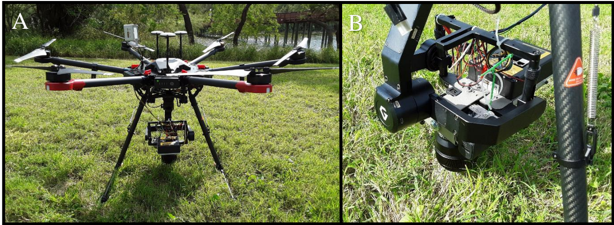
Figure 5. Drone and equipment used to conduct drone surveys for aquatic turtles. (A) DJI Matrice 600 Pro unmanned aerial vehicle with additional survey equipment attached; and (B) Gremsy T-3 gimbal with the SONY digital camera and MAIA multispectral camera attached.
