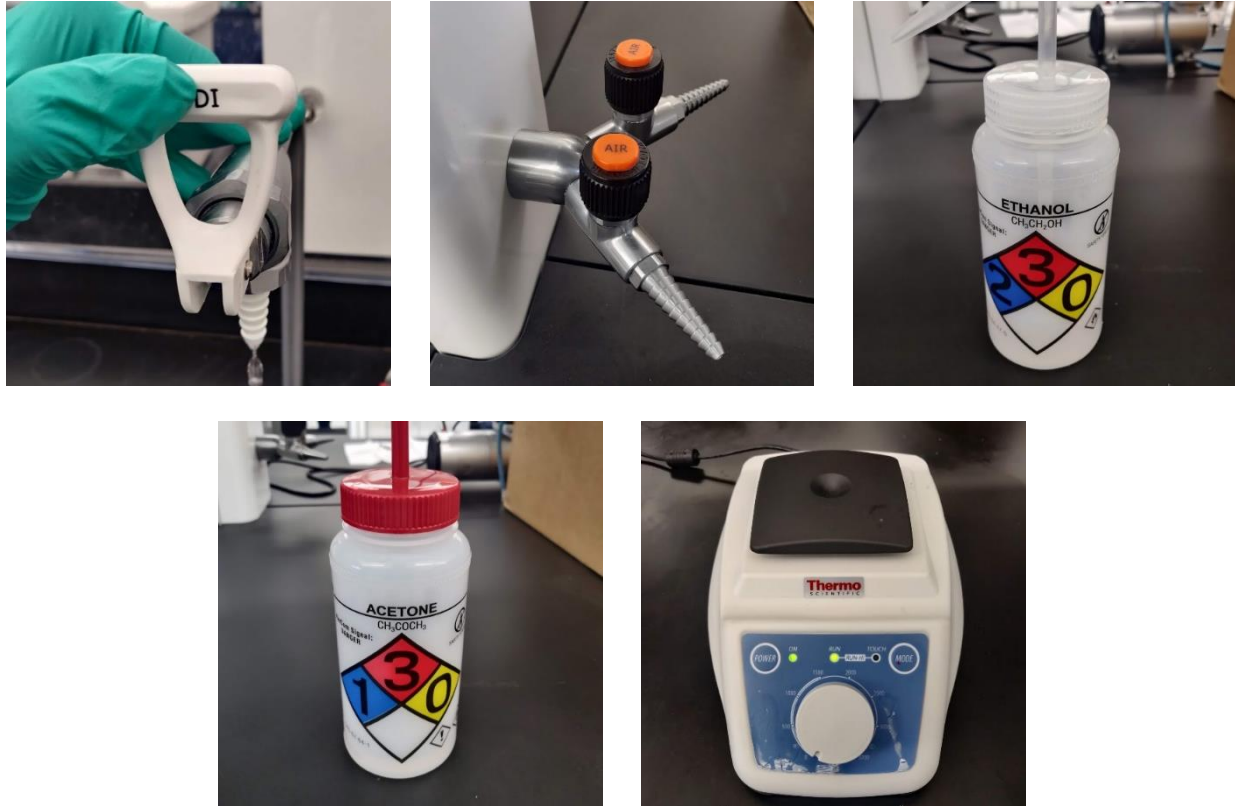
Figure 9: Cleaning steps (a)DI water (b) filtered air (c) ethanol (d) acetone (e) micromixer.
