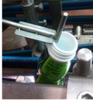
Figure 19 Flipper grabbing bottles
