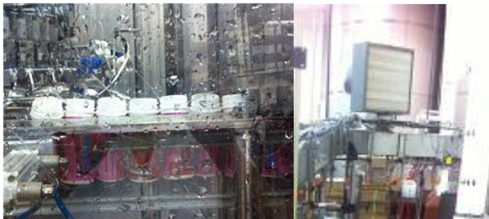
Figure 8 Bottles suspended in Air Conveyor
