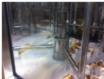
Figure 17 waste in star wheel
