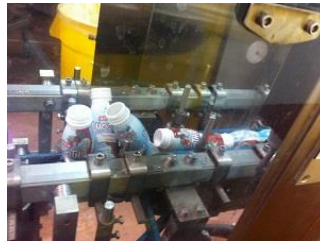
Figure 6 Bottles stuck in Descrambler
