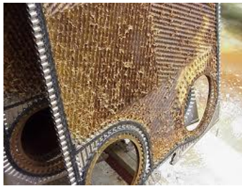
Figure 1 Fouling in heat exchangers
