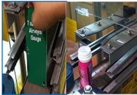
Figure 26 Air conveyor gauge
