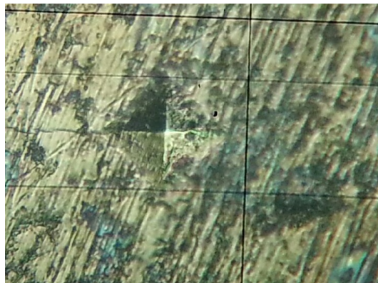
Figure 2.4: Hardness Test Indentation in Terfenol-D Sample
