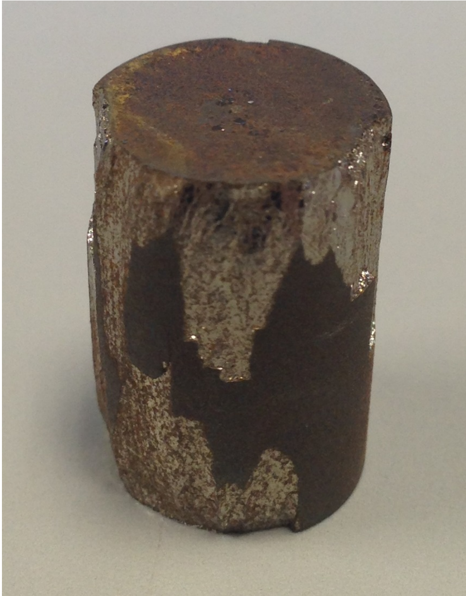
Figure 3.12: Terfenol-D Wear and Tear Caused by Lateral Loading
