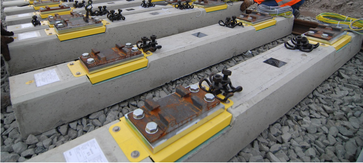
Figure 4.1: Load Cells in the Rail
