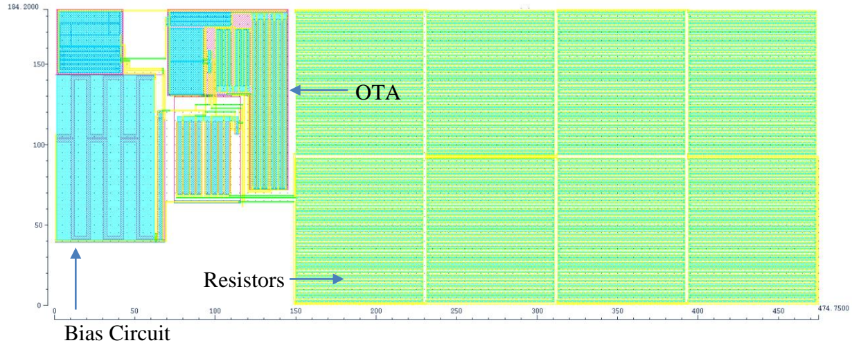
Figure 29. Amplifier Layout (including bias circuit) with an area of 474.75µm x 184.2µm
