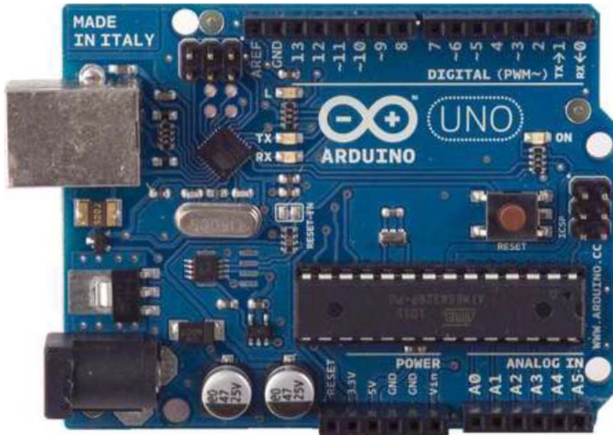
Figure 11: The Arduino Uno. Source: www.Arduino.cc
