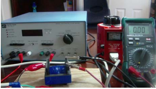
Figure 13: Transformer prepared for Short Circuit Test
