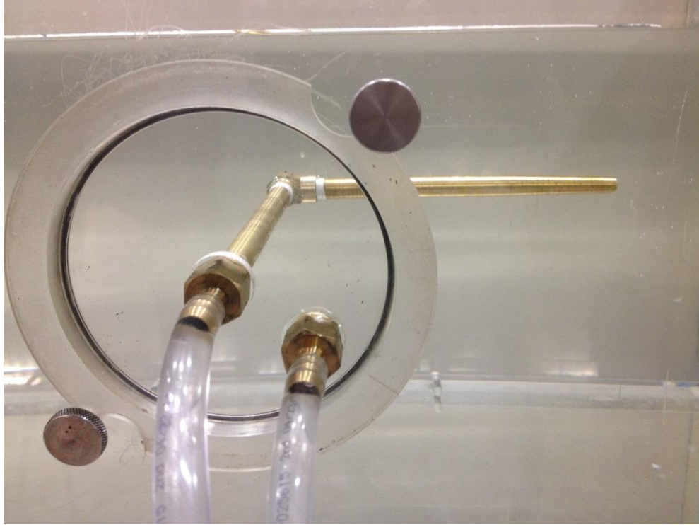
Figure 13. Pitot tube installed in water tunnel.
