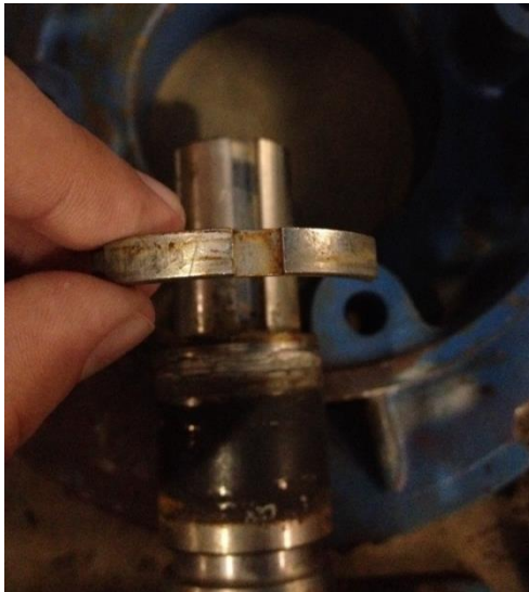
Figure 7. Fractured mechanical seal
