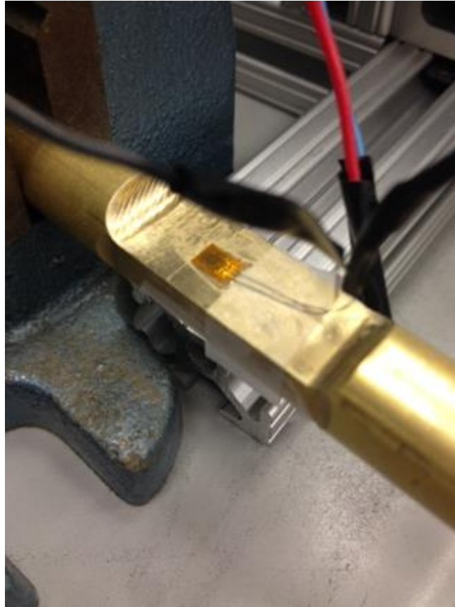
Figure 25. Strain gauge mounted on attachment cylinder.
