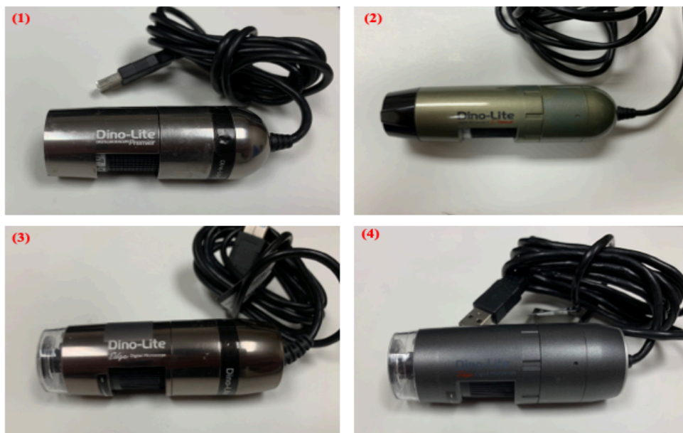
Figure 10 - Dino-Lite Digital Microscope Cameras. (1) Dino-Lite Premier, model number AM7013MZT with a 5-megapixel sensor, and maximum magnification of 200x. (2) Dino-Lite Premier model number AM4113TS with a 1.3-megapixel sensor capable of a maximum magnification of 220x. (3) Dino-Lite Premier Edge, model number AM7515MT89 with a 5 megapixel sensor, magnification from 700x to 900x and max resolution of 2592x1944, (4) Dino-Lite Edge, model number AM4515T8.
