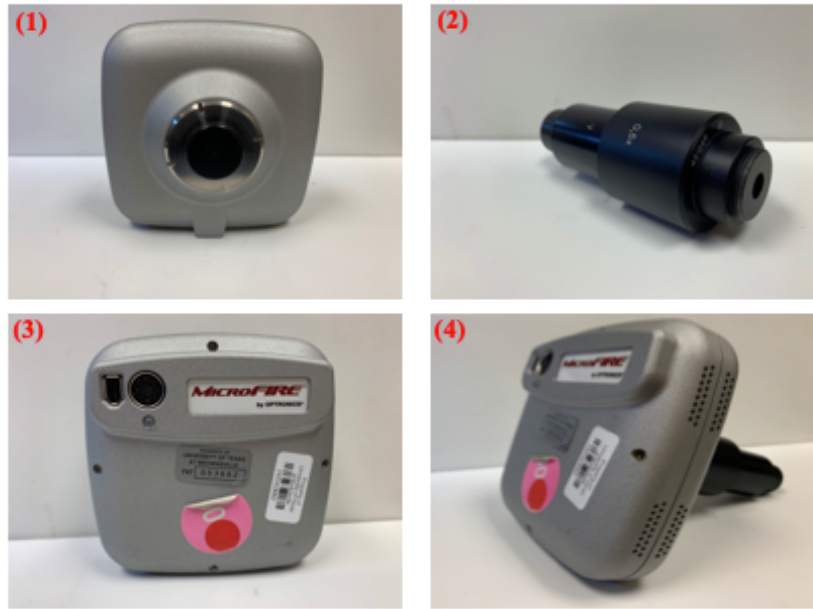
Figure 9 - Optronics Microfire camera. (1) Front view, (2) 0.5x C-Mount attachment, (3) Back view, (4) Optronics Microfire camera coupled with 0.5x C-Mount.
