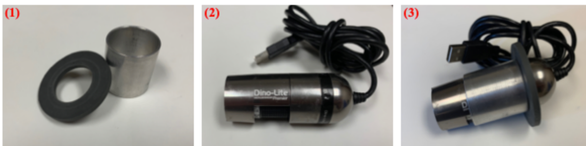
Figure 11— Set-up needed to fit a Dino-lite Digital Microscope Camera into the viewing port of the Axiovert 25 CFL Inverted microscope. (1) Aluminum sleeve developed by Mr. Antonio Suarez at the UTRGV machine shop for the Biophysics Research Lab, (2) Dino-Lite Premier, (3) Dino-Lite Digital Microscope Camera coupled with the aluminum sleeve and the rubber O-ring.
