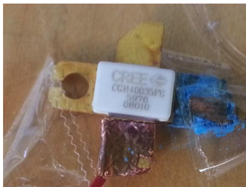
Figure 6.16 – HEMT used to obtain threshold data from the previous figure. Corrosion is obvious in this picture taken at around 8 months after experiment.
