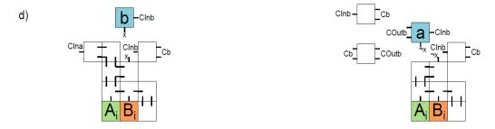
Here we see that if the input values are equal, the carry that was just generated will be sent to the next block immediately. However, if the input values are not equal, the carry for next block will be propagated after the carry-in is accepted.
