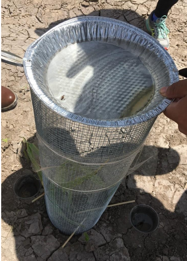
Figure 3.S3. Picture of unique three trap cage set up enclosing Sorghum-sudangrass ( Sorghum x drummondii ) in the field to collect attracted insect community.
