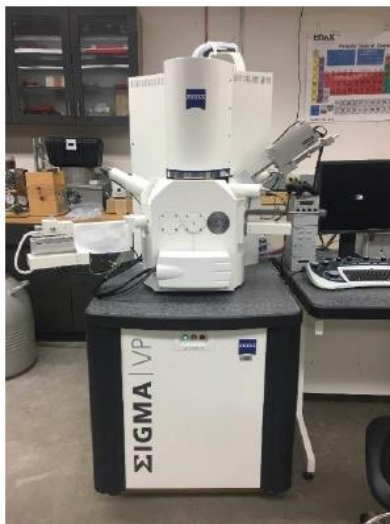
Fig. 29. Zeiss Sigma VP SEM equipment [58].
