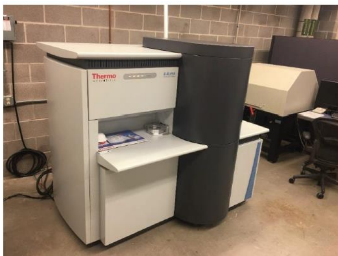
Fig. 30. Thermo Scientific K-Alpha XPS equipment [58].
