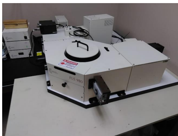
Fig. 33. Edinburgh Instruments FLS980 Fluorescence Spectrometer (PL) Equipment.
