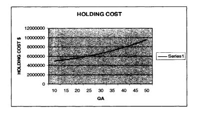
Figure 4.20 Holding Cost plot for fix  $Q_B$  and varying  $Q_A$  for higher production rate for both the products.
