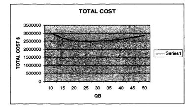
Figure 4.16 Total Cost plot for fix  $Q_A$  and varying  $Q_B$  for higher production rate of higher priority product.
