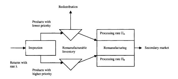
Fig 3.1 Schematic diagram of Production System in Reverse logistics
