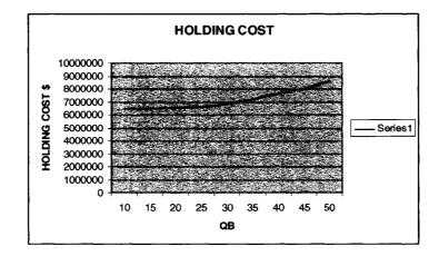
Figure 4.17 Holding Cost plot for fix  $Q_A$  and varying  $Q_B$  for higher production rate of higher priority product.
