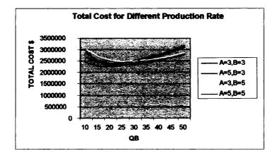
(b) A sensitivity analysis of total cost for different production rate is shown in figure 4.26
