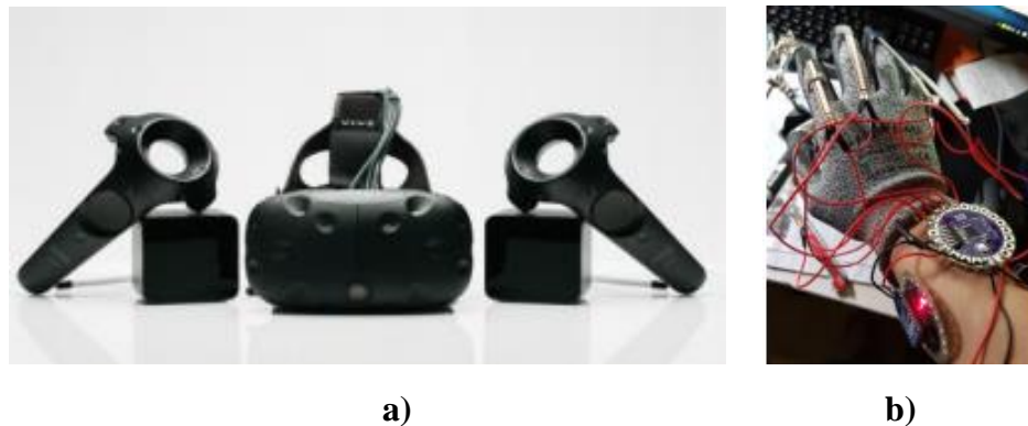
Figure 2.13 Controllers; a) HTC Vive equipment; b) Data Glove [26].
