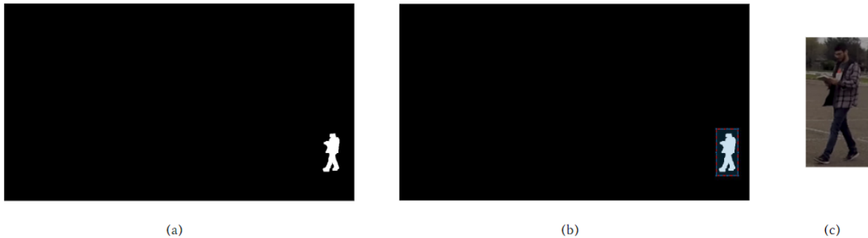
Figure 2.3: Example of pseudo ground truth bounding boxes: (a) a foreground mask for a frame in a sequence, (b) the bounding box coordinates from that frame, (c) the resulting crop from those bounding box coordinates.
