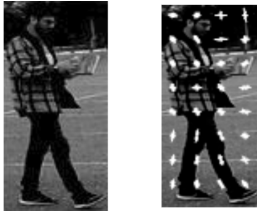
Figure 3.2: HOG features on one custom data crop with 15x15 masks.
