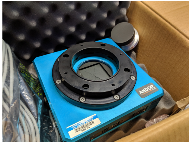
Figure 3.9: Apogee Alta F16M being prepared for mounting onto CDK17
