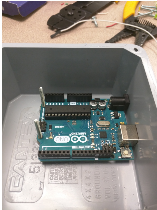
Figure 3.3: Arduino Uno inside enclosure
