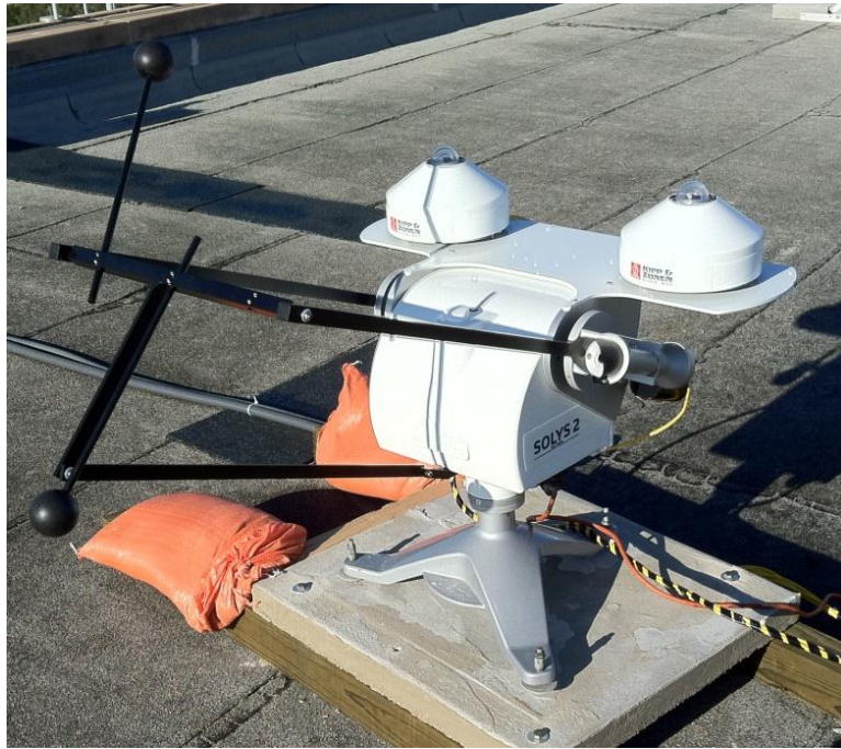
Figure 3.3 – Solar Radiation Lab. Two pyranometers, one pyr heliometer, and the tracker
