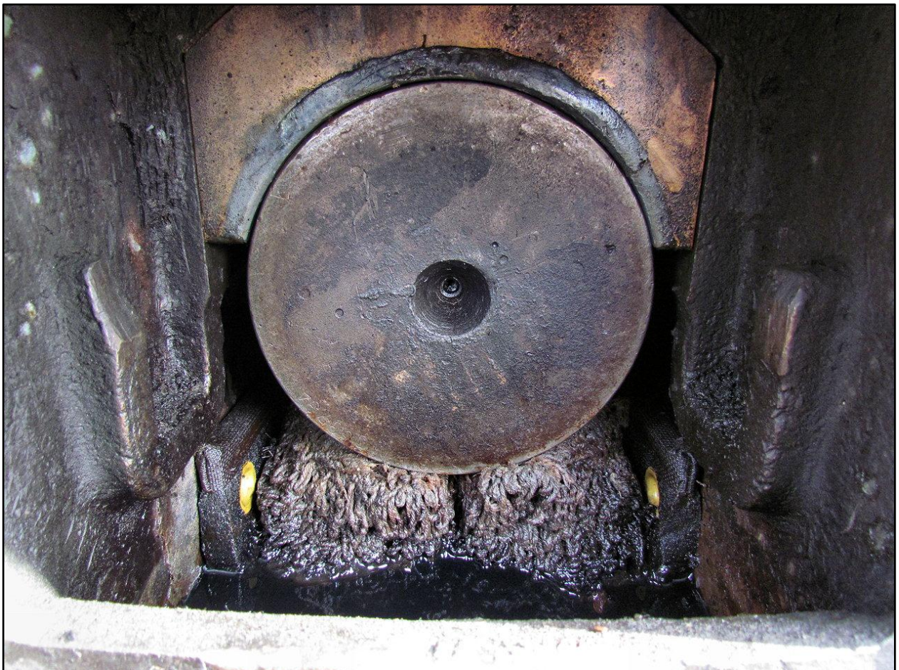
Figure 3: Enclosed railcar axlebox with plain bore journal bearing [15]
