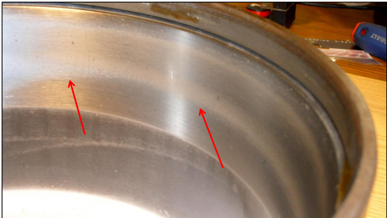
Figure 30: Detailed view of one raceway of the L3 bearing cup with the varied width of the wear pattern indicated.
