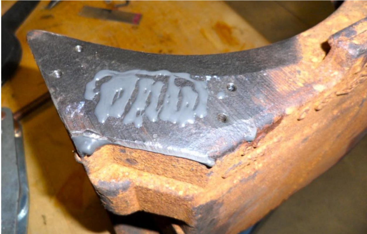
Figure 14: Primed mounting surface with the thermal epoxy and mounting holes shown [12].
