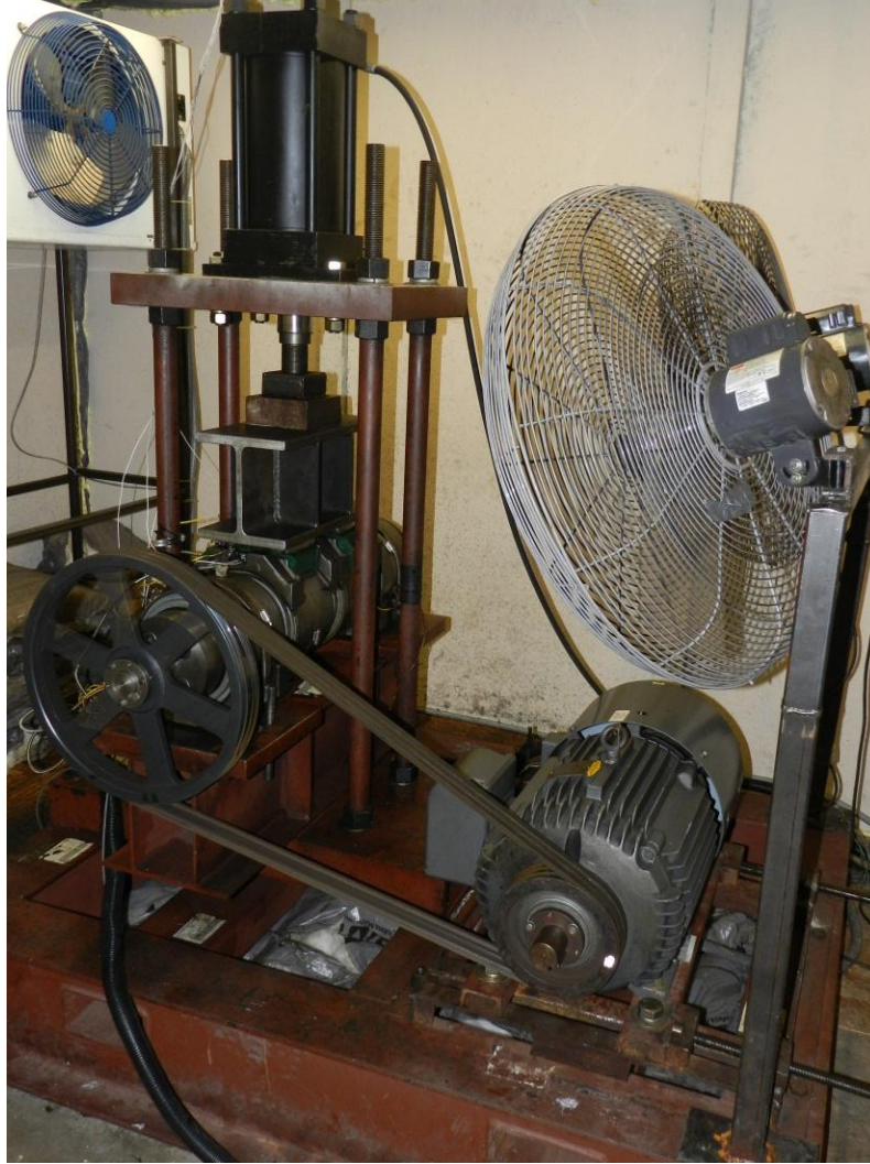
Figure 17: Dynamic bearing tester used for laboratory experiments conducted at UTPA
