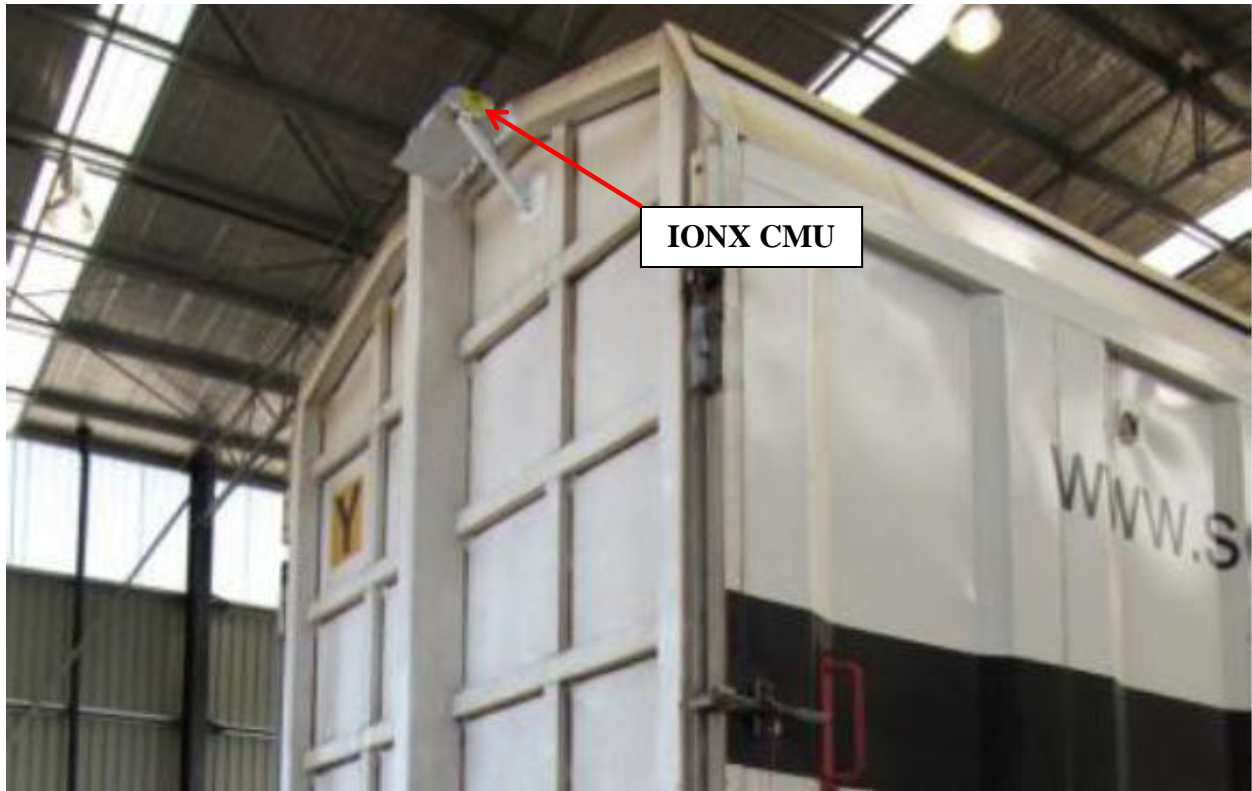
Figure 16: Field installation of IONX CMU on a freight car [28]
