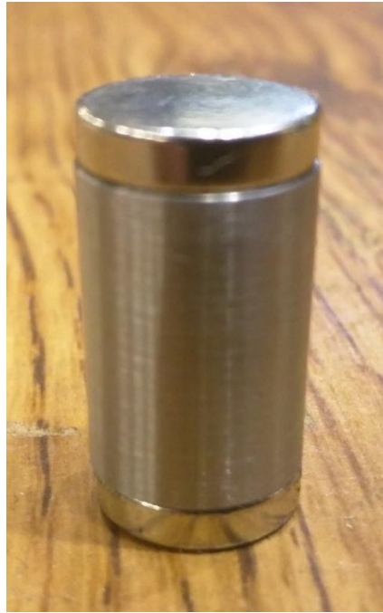
Figure 3. Terfenol-D rod with 3300 Gauss neodymium magnets.
