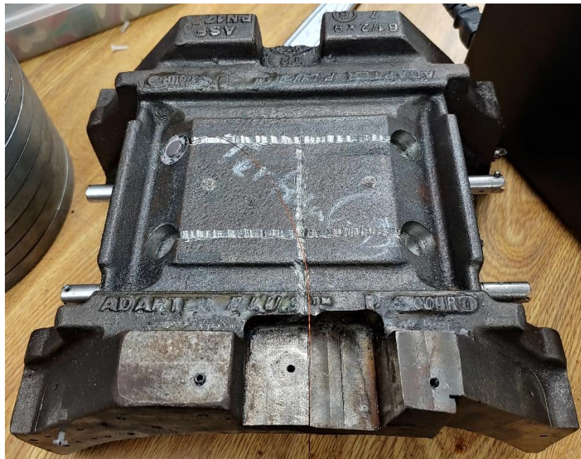
Figure 27. Machined channels providing an exit for the coil leads.
