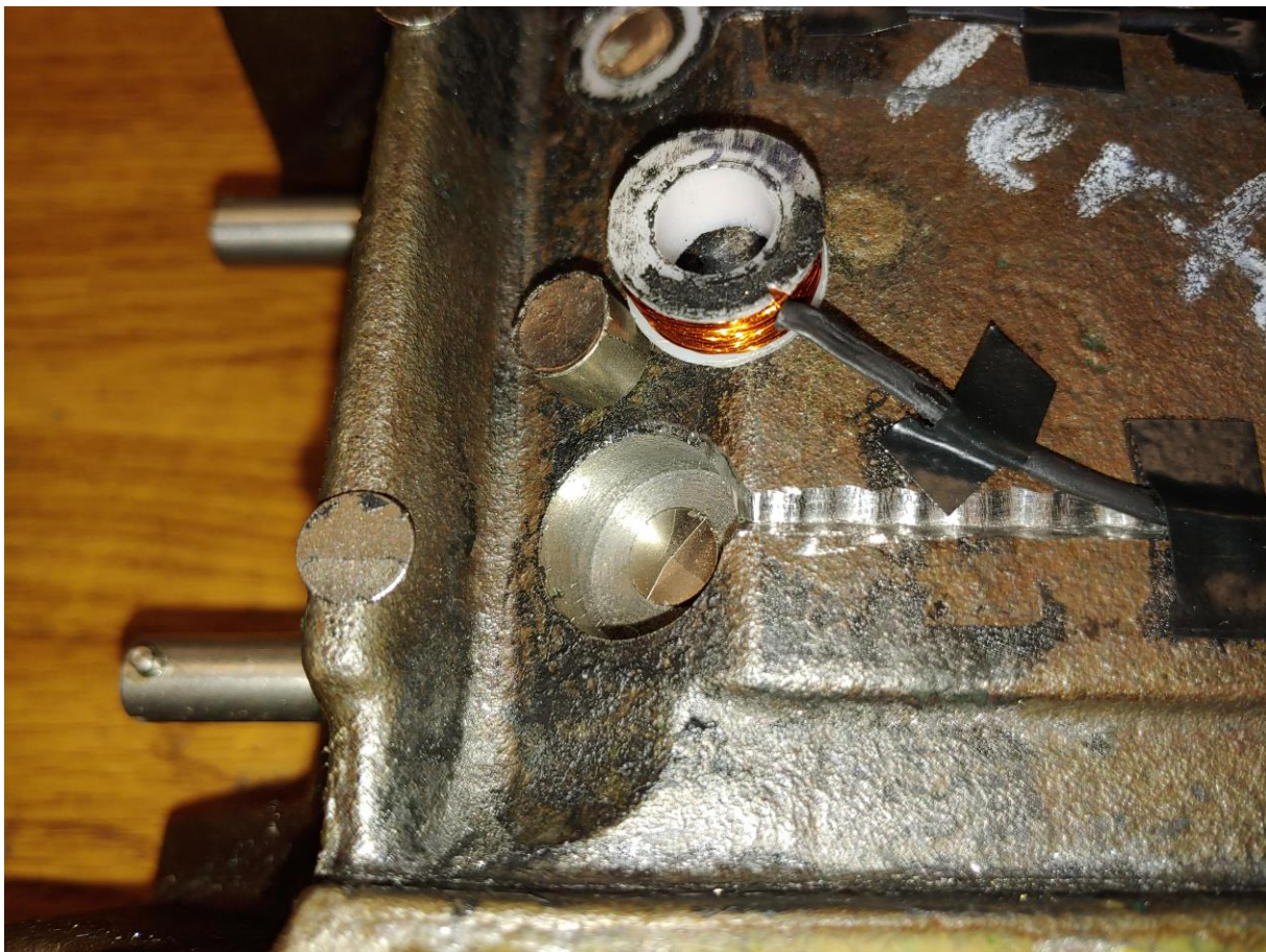
Figure 44. Post-test damage to magnets.
