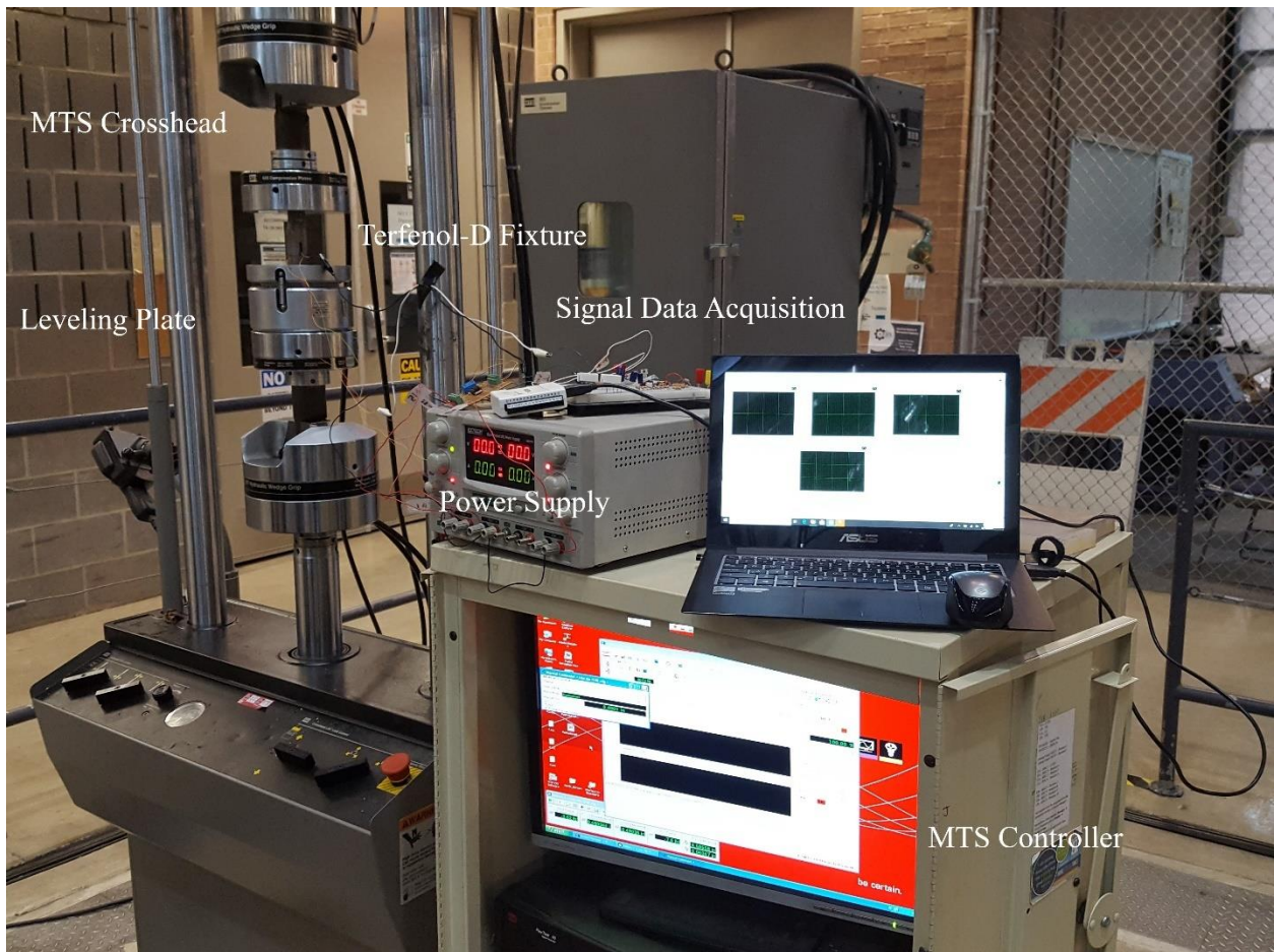
Figure 2. Material Test System (MTS) with instrumentation.
