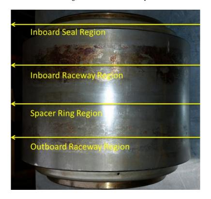
Figure 9. Infrared scanning locations on the bearing
