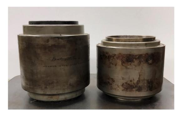
Figure 3. Class F (pictured left) and Class K (pictured right) bearings
