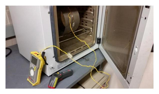
Figure 19. Oven test experimental setup [19]
