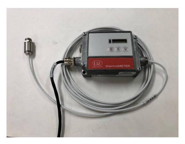
Figure 16. MICRO-EPSILON infrared (IR) temperature sensor
