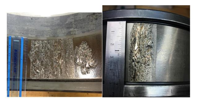
Figure 18. Outer ring (cup) spall from Exp. 198C (pictured left) and inner ring (cone) spall from Exp. 202A (pictured right)
