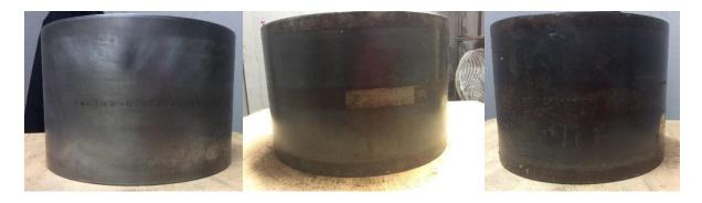
Figure 21. Examples of bearing cups used for emissivity testing includes brushed surface (left), moderately used surface (center), and heat-tinted rusted surface (right)
