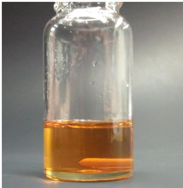
Figure 10: Dissolved microcrystalline cellulose in 1-ethyl-3-methylimidazolium acetate and dimethyl sulfoxide (DMSO).
