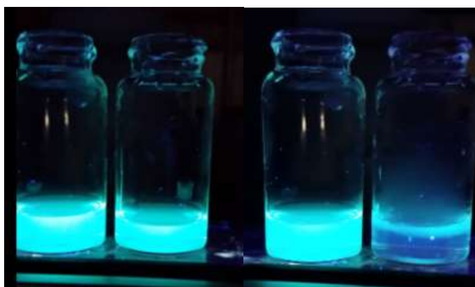
Figure 3.12: Quenching of luminescence after the addition of HCl because of the protonation of the amine group.
