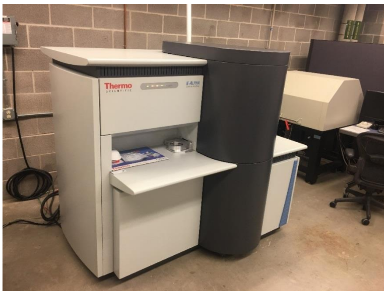
Figure 12 - The XPS was used to measure the elemental composition of the fibers.
