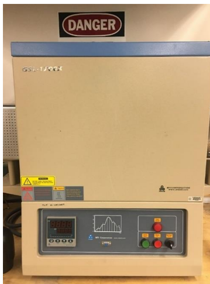
Figure 17 – GSL – 1700X used to carbonize PVA-Pb fiber mats.
