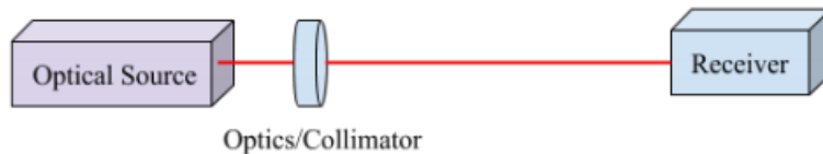
Figure 2.2: Scheme of a basic free space optical communication link.
