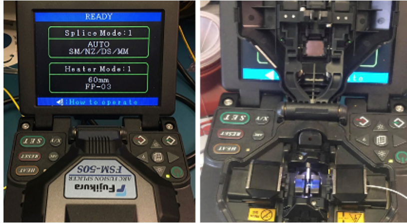
Figure 5.5: Fujikura Fusion Splicer FSM-50S. Right picture: The ends of the fiber cables are aligned within the splicer before fusion.
