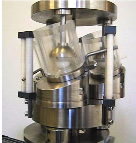
Figure 2.9. – Hip Joint Simulator With Biaxial Reciprocating Motion (BRM), HUT – 3.
