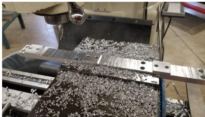
Figure 4.2. – Aluminum Piece, Manufactured On A Milling Machine.
