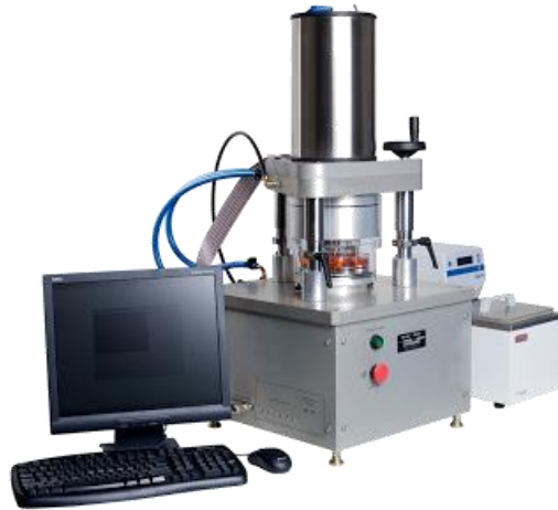
Figure 2.8. – Orthoped Tribometer Developed By AMITI.
