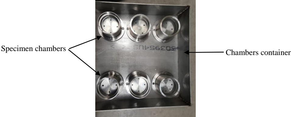
Figure 4.8. – Specimen Chambers Mounted On The Chambers Container.
