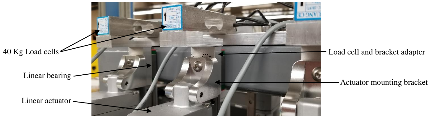
Figure 4.9. – Load Cell Mounted Above The Linear Actuator.
