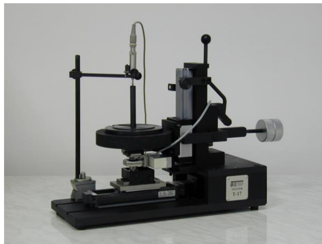
Figure 2.6. – Reciprocating Tribometer Model T-17 From The Institute For Sustainable Technologies.
