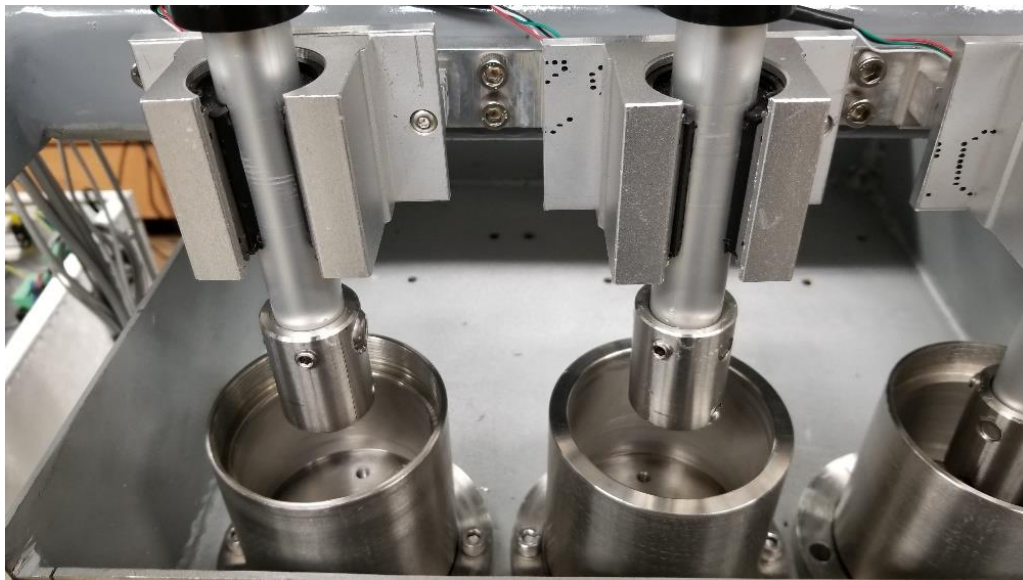
Figure 4.13. – Pin Holder Installed On Each Linear Actuator.
