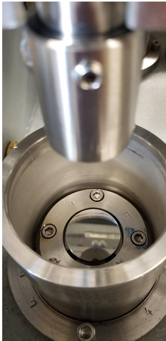
Figure 4.21 Specimen Mounted On The CNC-POD Before The Wear Tests.
