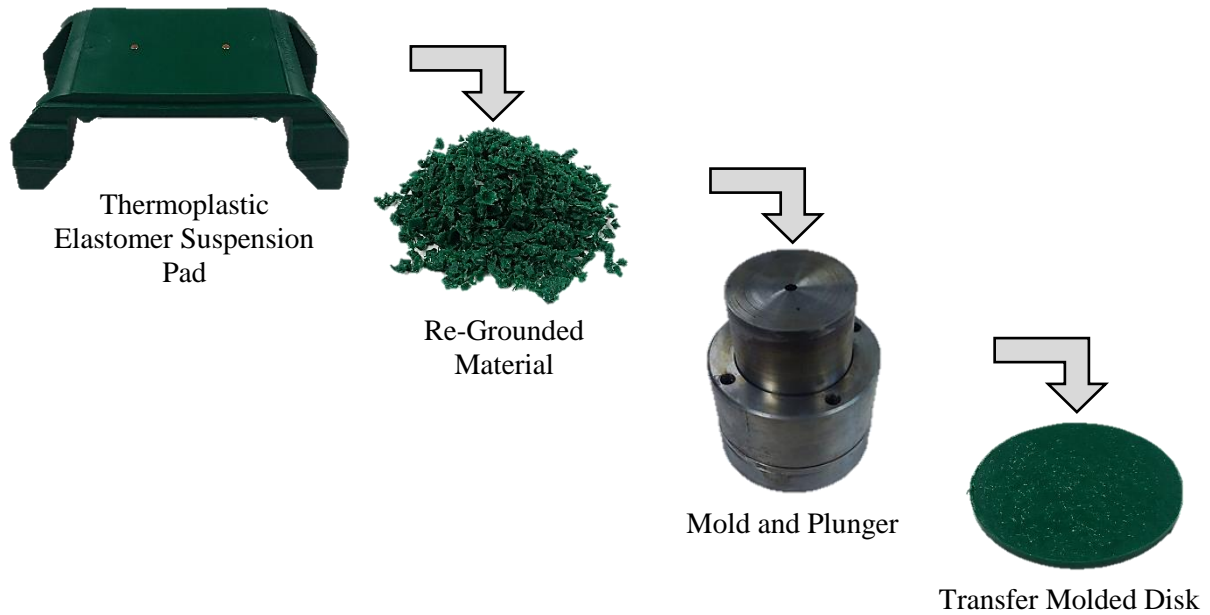
Figure 2.6. Transfer molding process for DMA sample preparation.
