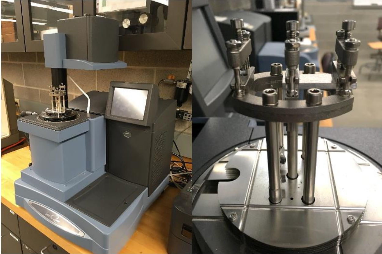
Figure 2.5. TA Instruments Q800 Dynamic Mechanical Analyzer (DMA) (left) and single cantilever configuration setup with calibration sample (right).
