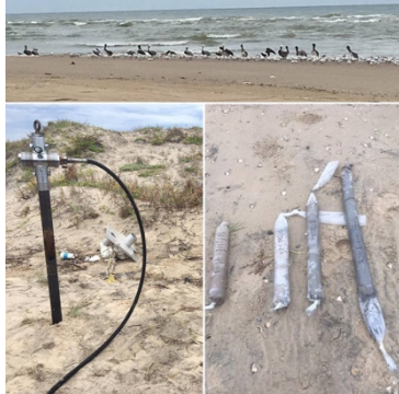
Figure 15 Boca Chica Beach. Top picture is of the Gulf of Mexico. Bottom left is of the Vibracore and sand dunes. Bottom right- core samples from the Vibracore near the mouth of the river at Boca Chica Beach.
