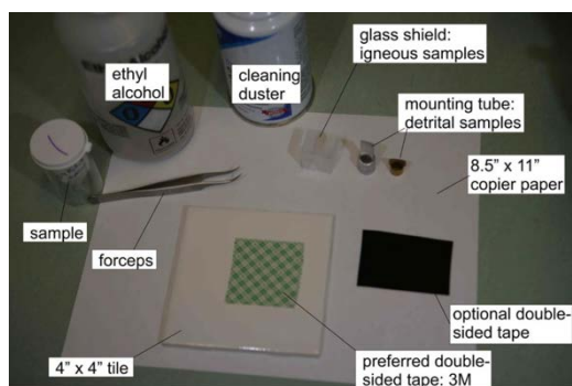
Figure 17 Materials needed to mount the samples. Photo courtesy of Pullen and Pepper, 2009
