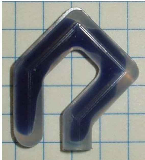
Figure 20. PP Sample fabricated under the optimum processing conditions showing the gas penetration.
