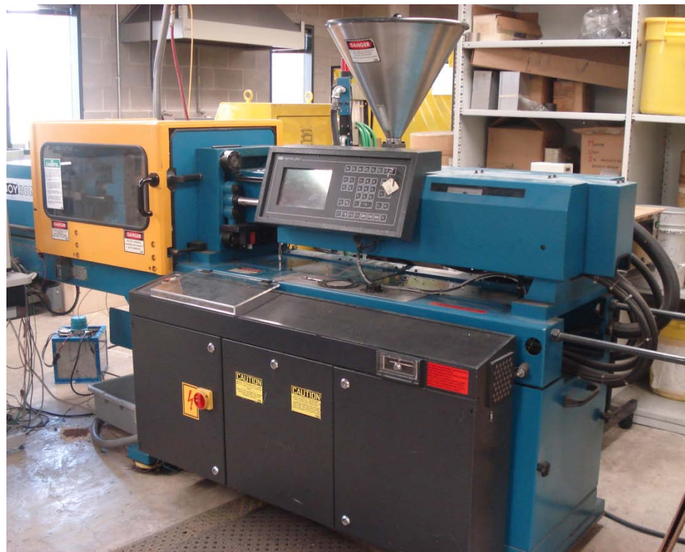
Figure 8. Boy 30M injection molding unit.
