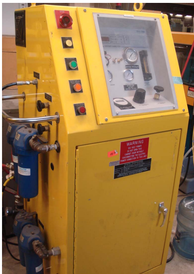
Figure 9. Gain Technologies nitrogen generator.
