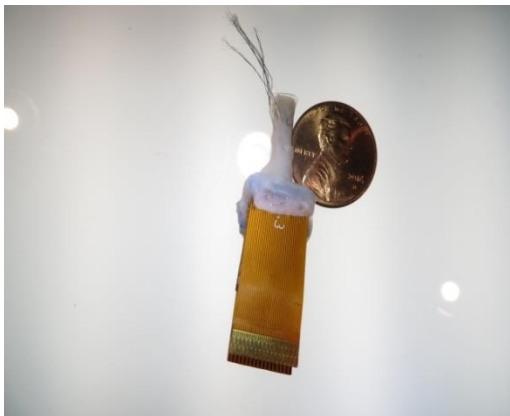
Figure 2.11: ECoG Device with dental cement in two views
