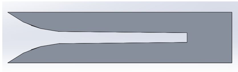
Figure 54: Anchor Lock with Wide Opening
