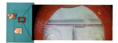
Figure 6: Orthogonal electrode pair on a PDMS coated glass slide
