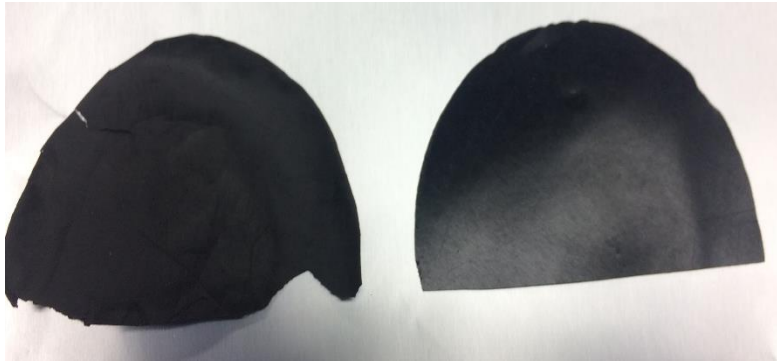
Figure 14. (a)CNF mat, left. CNT/PP composite, right
