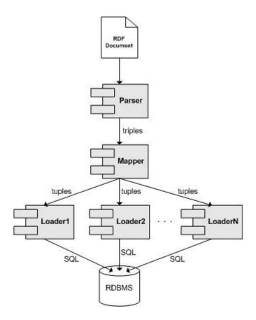
Figure 9: Data Mapping Architecture of S2ST
