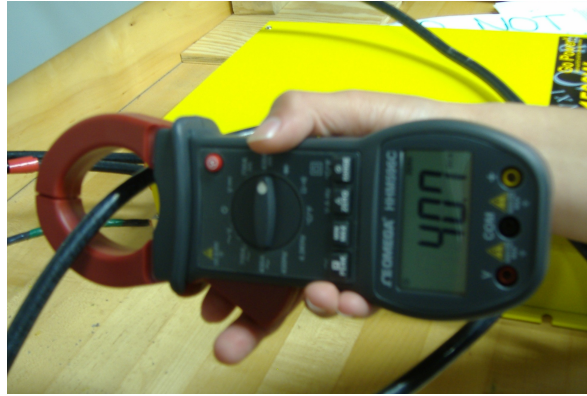
Figure 25: Calibration of the Current Transducer I_L with a Clamp Meter
