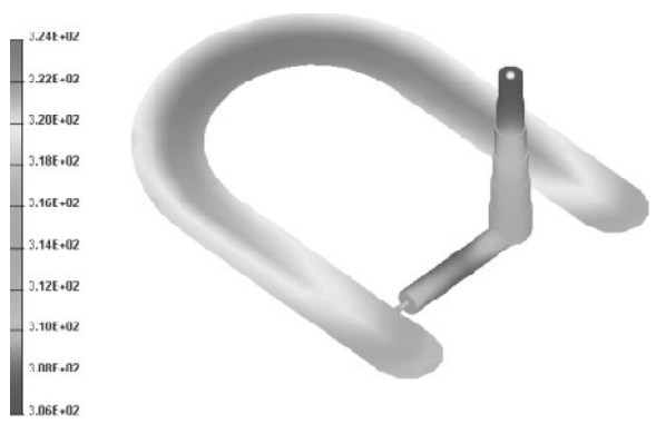
Figure 2- 5: Simulation Analysis showing average mold cavity wall temperature distributions [34]
