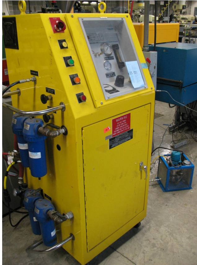
Figure 3- 8: GAIN Technology Nitrogen Generator
