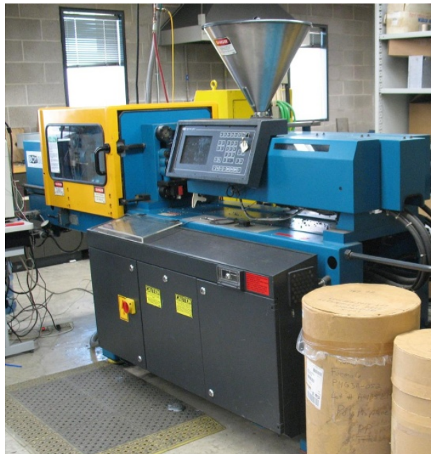
Figure 3- 7: Injection Molding Machine BOY 30M
