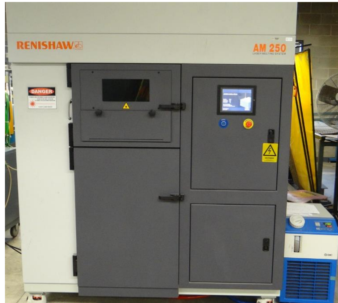
Figure 3.2- Renishaw AM 250 laser melting machine
