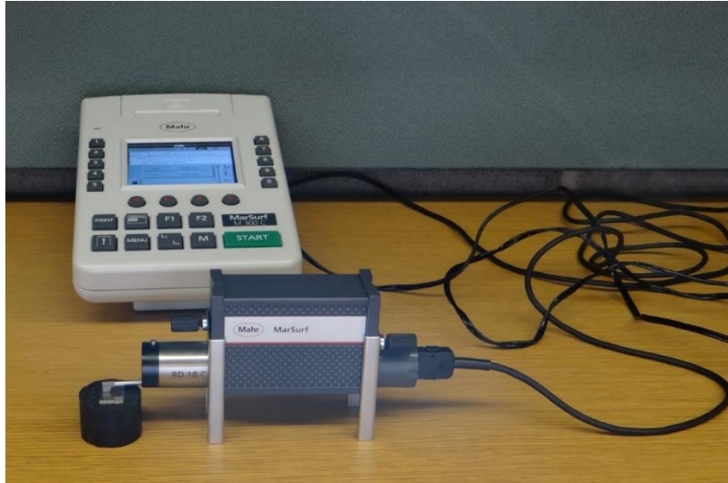
Figure 3.12- roughness measuring instrument set up
