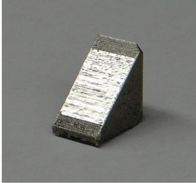
Figure 3.4- Typical SLM printed sample based on Box-Behnken design
