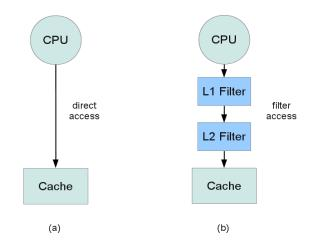
Figure 3.4: (a) Conventional Cache Architecture. (b) Two-Level Filter Cache Architecture.
