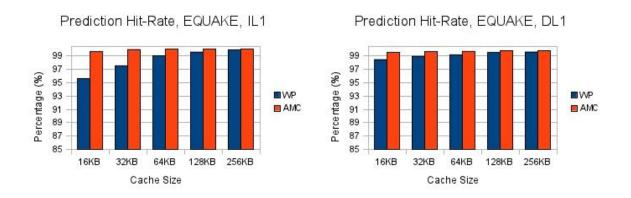
Figure 6.30: Prediction Hit-Rate for EQUAKE Benchmark
