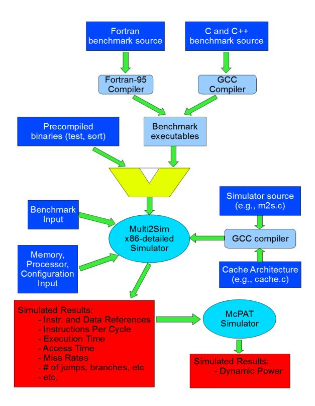
Figure 5.2: Multi2Sim Simulation Model
