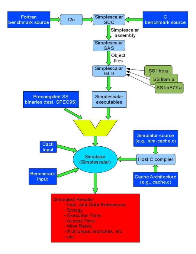
Figure 5.1: Simplescalar Simulation Model
