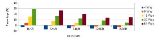
Figure 6.17: Results for EQUAKE Benchmark
