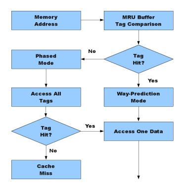
Figure 4.1: BCC Cache Access Mode Sequence
