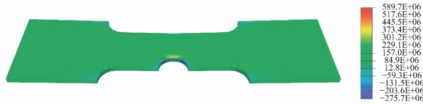
Figure 7: Distribution of \sigma_{22} stress tensor component (along the loading direction) after tension with the loading equal to 10 kN.
