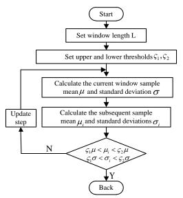
Fig. 2. Algorithm flow of real-time moving window
