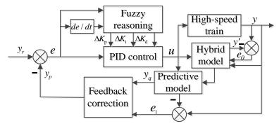
Fig.4. Diagram of predictive Fuzzy PID control system
